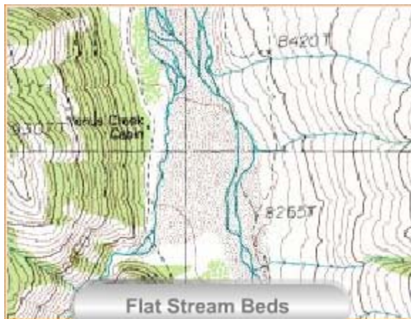
Caption: An example of a flat stream bed as indicated on a topographic map.
