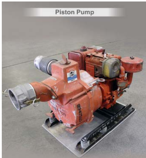
Caption: An example of a piston pump.
